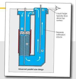
Isotech baths are purpose designed for thermometer calibration with cylindrical calibration volumes of good depth. Compared to other large rectangular designs Isotech baths require less fluid for the same depth and can offer significant initial and on-going cost savings.
