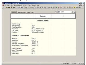
The MadgeTech algorithm has been validated against the United States Pharmacopeia (USP) and will yield a value within 0.1°C for all inputs. It is also important to note that the MadgeTech software uses constants that are more recent and marginally more accurate than the USP. MadgeTech obtains these constants from the CODATA/ NIST recommended values.
