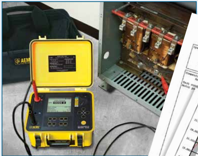
Model 6555 performing insulation test.
