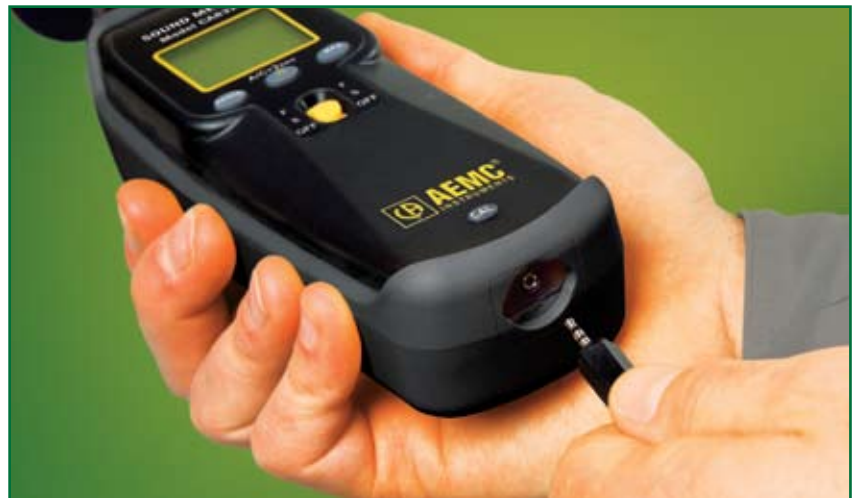
The Model CA832 includes an auxiliary output for connecting the instrument to a recording device.
