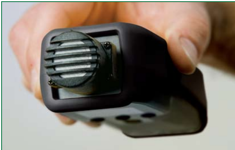
The Model CA895's catalytic sensor does not consume any chemical substances.
