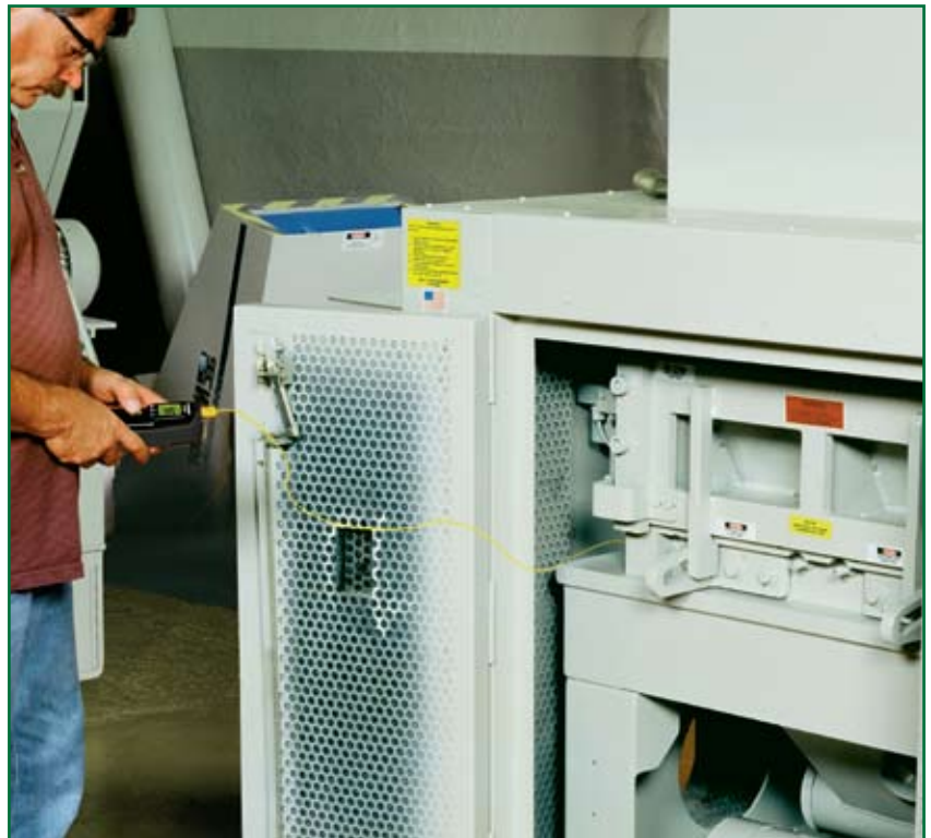
Temperature measurement on industrial oven used in reclaiming defective plastic parts
