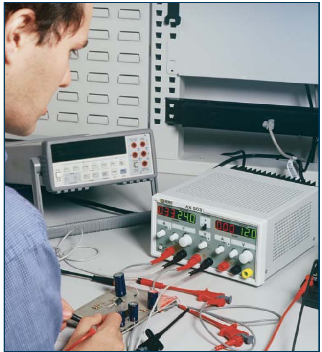
Circuit board design testing using the 30V and 5Vdc outputs
