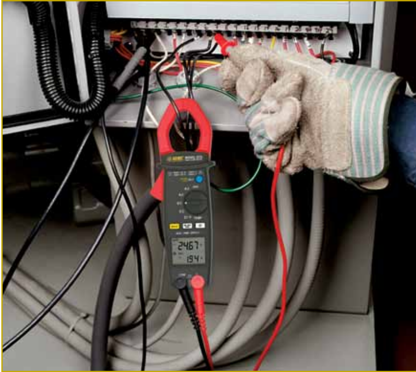
Model 675 measures both volts and amps and displays results simultaneously.
